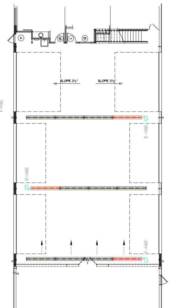
IRH-1 ROTATE REFLECTOR IN DIRECTION OF ARROWS. THIS HEATER CAN ALSO BE PLACED TO THE FAR LEFT INSTEAD.
